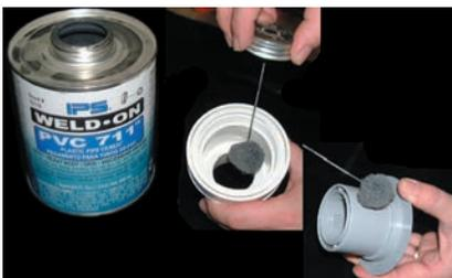
Use any PVC/PVC glue on Pool Valet body in pool and on Pool Valet Retro body to be installed.
